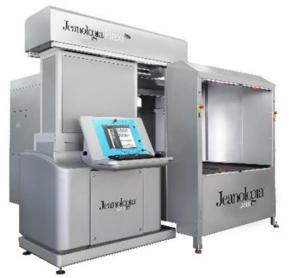
We use Laser Technology from Jeanologia to replace manual whiskering process, hand sanding and PP spray and rips and damages, thus reducing hazardous health impact of our workers.
